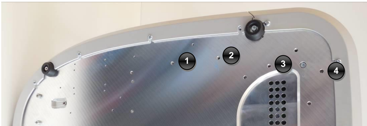
Fig. 14 – Instrument bottom with holes for tablet and joystick supports
