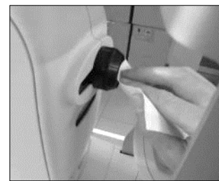
Figure 67 – Clean the lens
