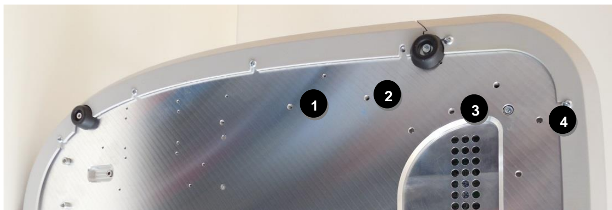
Fig. 12 – Instrument bottom with holes for tablet support bracket
